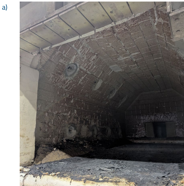
Figure 7: (a) Inside of a car-bottom furnace; notice eight burner holes in the refractory lining and significant scale on the floor. (b) Electric manipulator removing steel workpiece from furnace.
